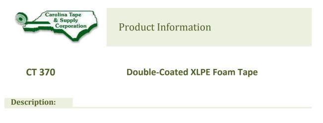
1/32" thick, cross-linked white polyethylene foam tape with high tack and high shear with a synthetic rubber adhesive. Available in other thicknesses.
